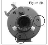
Figure 5b: Now, with the 3mm Allen wrench turn the two adjacent large screws *clockwise* no more than 1/4-turn.
