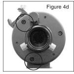
**Figure 4d:** Turn the two large screws adjacent to the small screw *counterclockwise* no more than 1/4 turn.
