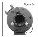
Figure 5a: Using the 2mm Allen wrench, turn the large screw counterclockwise a small amount, no more than 1/4 of a turn. (Note: Actual selected alignment screw will vary.)
