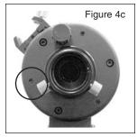
**Figure 4c:** Turn the small screw that is 180° opposite the first screw *clockwise* no more than 1/4 turn.
