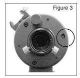
Figure 3: If the view through the rear opening of the telescope resembled Figure 2a, then the alignment screw you would start with would be this one. The actual first alignment screw you would pick will vary depending on which way the front opening would need to move in order to "fill" the black crescent.
