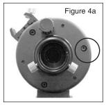
Figure 4a: Using the 3mm Allen wrench, turn the large screw *clockwise* a small amount, no more than 1/4 of a turn. (Note, actual selected alignment screw will vary.)
