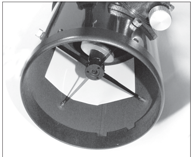
Figure 10. Placing a piece of white paper inside the optical tube opposite the focuser provides a bright background when viewing into the focuser.
