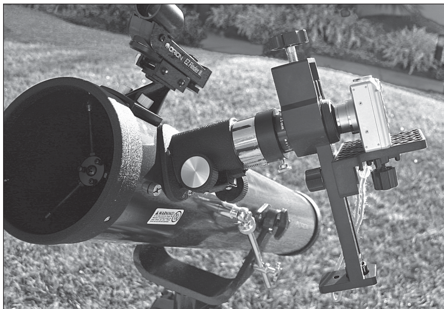
Figure 3. The SteadyPix Pro with camera attached is shown mounted on an Orion SpaceProbe 3 reflector telescope.
