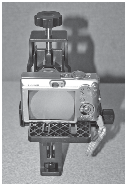
Figure 2. Camera position relative to the telescope eyepiece should be adjusted until the image covers as much of the LCD screen as possible.
