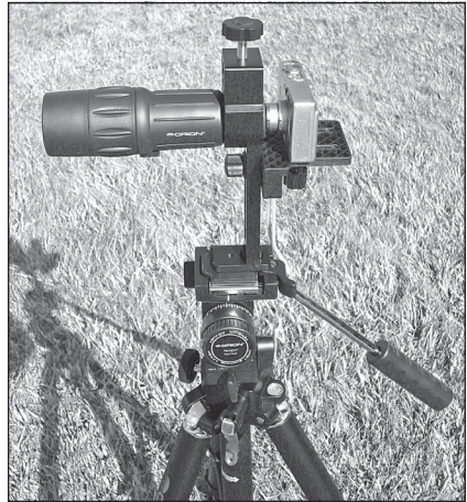
Figure 8. The SteadyPix Pro is shown attached to a photo tripod via the \frac{1}{4} "-20 socket in the SteadyPix's foot. A monocular is held in the eyepiece clamp.
