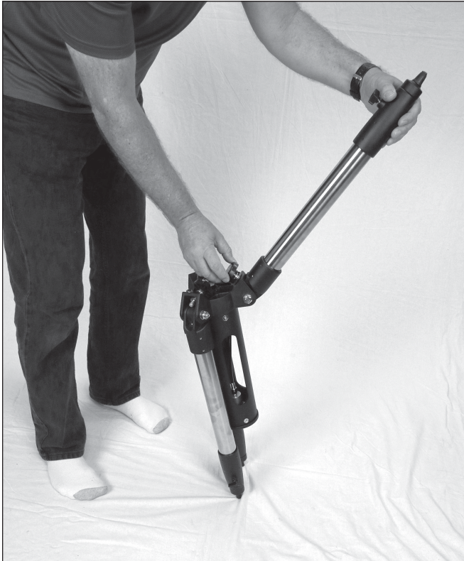
Figure 3. Fold the tripod legs down and lock each one with the captive rosette knob.
