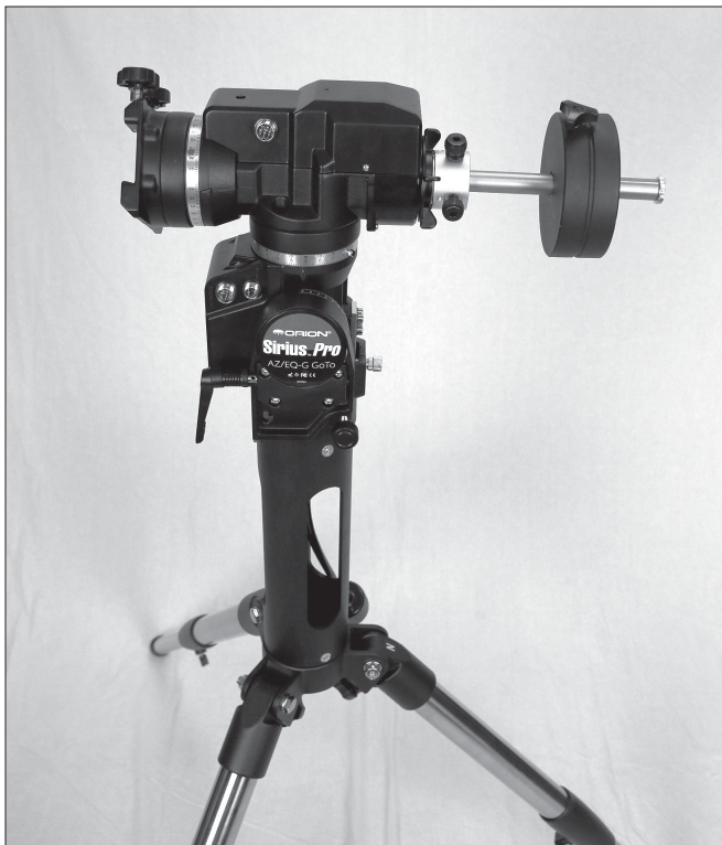
Figure 17. All set for single scope use in altazimuth mode.
