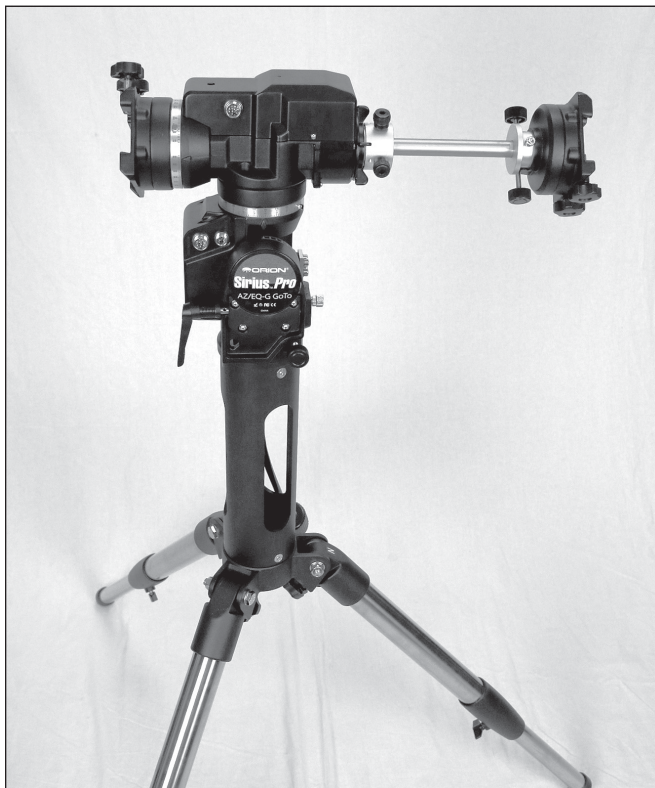
Figure 20. The mount is ready for installation of two telescopes.
