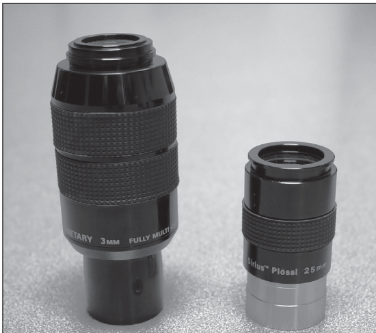
Figure 2. Examples of two eyepieces with housing diameters that are compatible with the SteadyPix EZ. The 25mm Sirius Plossl (right) has a housing diameter of 35mm; the 3mm Edge-On Planetary eyepiece has a housing diameter of 45.5mm. Both eyepieces are shown with their rubber eyecups removed.
