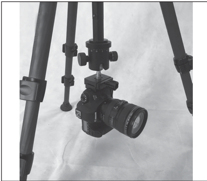
Figure 6. A camera and ball head mount (not included) are shown mounted on the secondary mounting platform, to get low to the ground.
