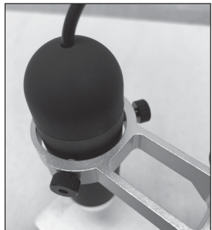
Figure 9. Drop the microscope down through the ring, and gently tighten down the two clamping screws.
