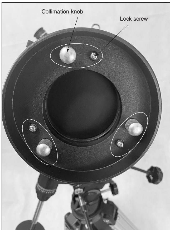
Figure 23. The tilt of the primary mirror is adjusted using the three pairs of collimation knobs and lock screws on the back end of the optical tube.
