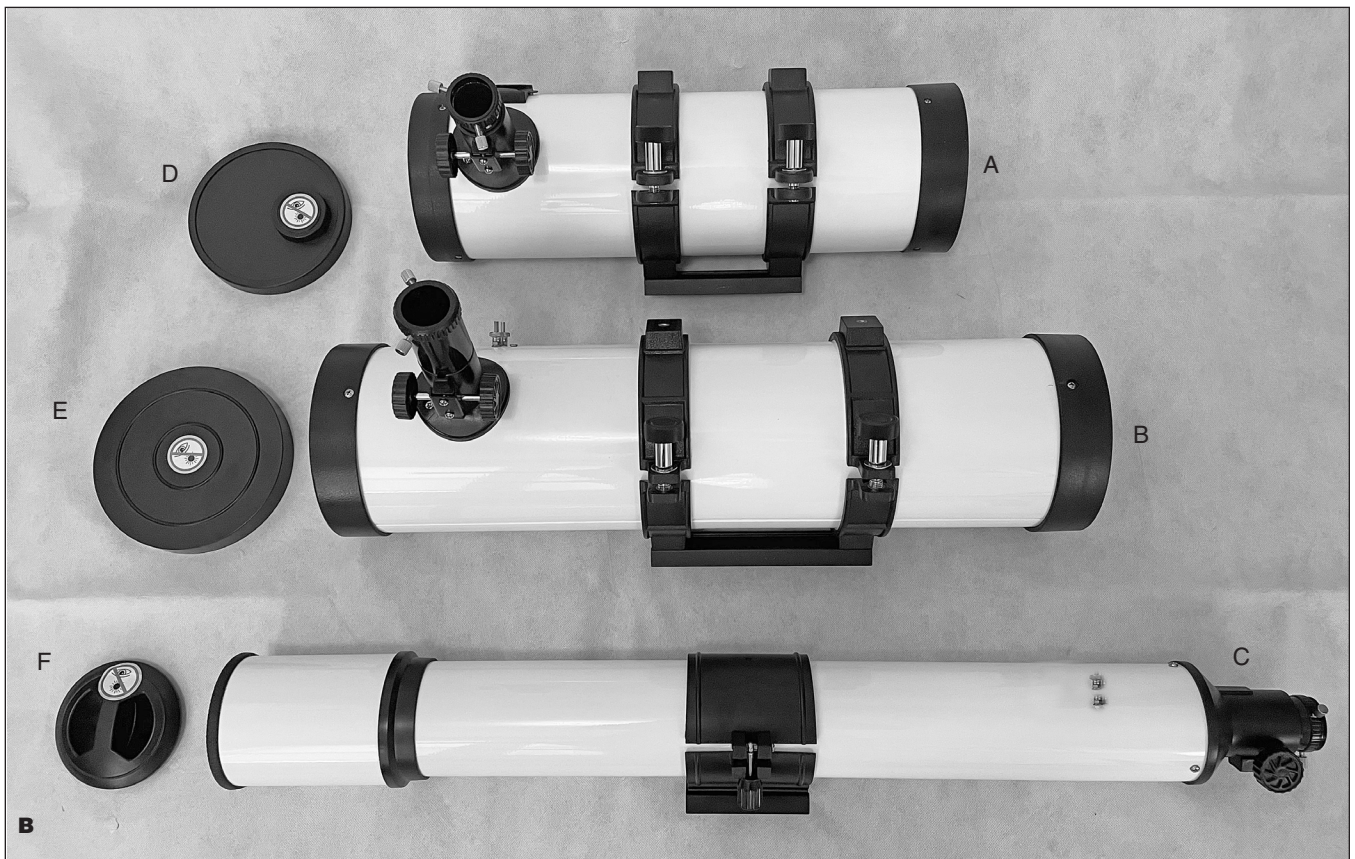
Figure 1. A) Parts included with the Orion Observer EQ telescopes. B) Optical tube assemblies of the Observer EQ telescopes.
