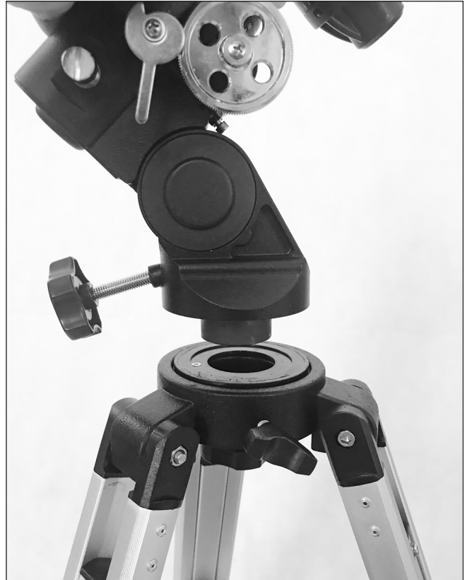
Figure 4. Place the equatorial mount on the tripod.
