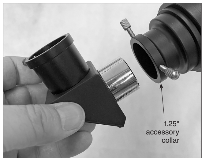
Figure 9. Insert the chrome barrel of the star diagonal into the 1.25" adapter's accessory collar, then secure it with the two thumbscrews.
