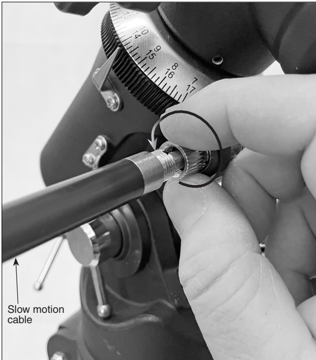
Figure 5. Attach the two slow-motion cables to the mount.
