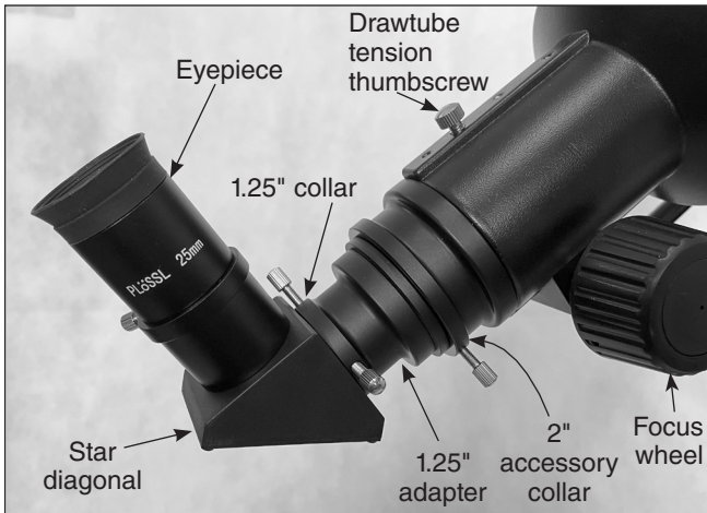
Figure 10. Insert the eyepiece into the star diagonal and secure it with the thumbscrew.
